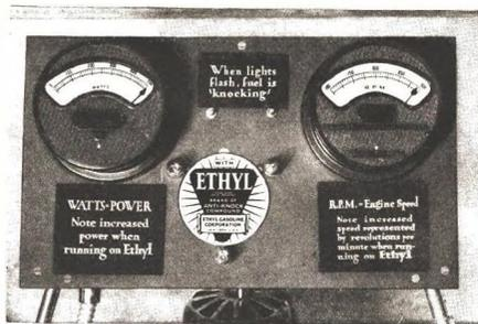
Left: When the lower picture was taken, Ethyl had been fed into the carburetor. The wattmeter shows that the power has risen to the maximum; the tachometer shows a corresponding increase in revolutions per minute.
